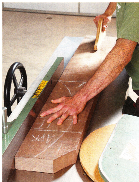
Press down and push. Use your left hand to keep the board flat on the jointer's table while pushing it forward with your right hand.
