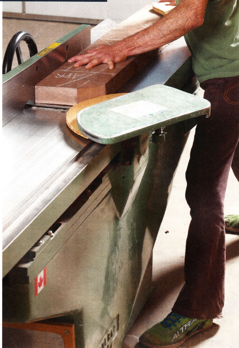
Press down and push. Use your left hand to keep the board flat on the jointer's table while pushing it forward with your right hand.
